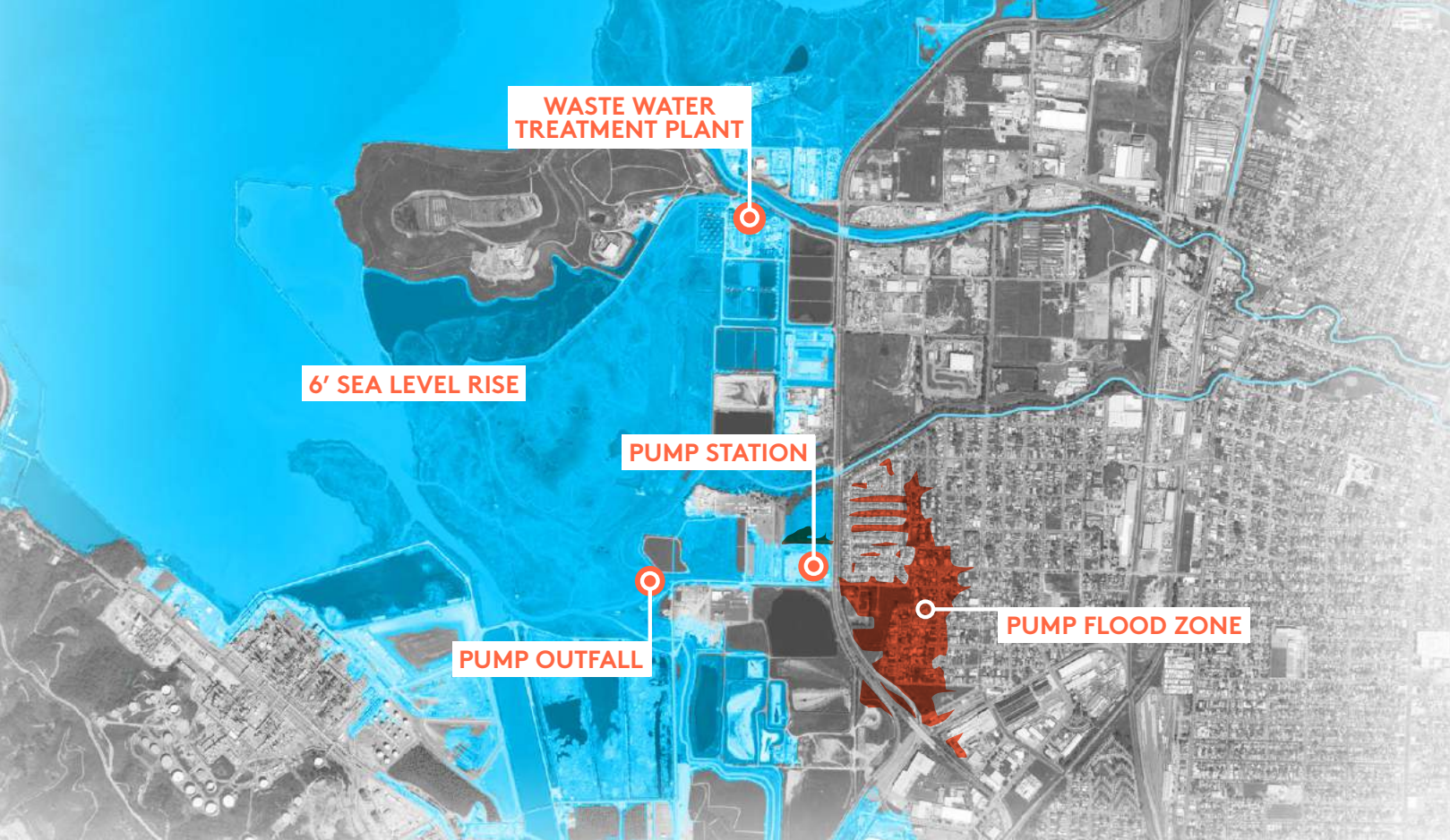
Above—Pump & SLR map: an aging pump and outfall lie within the 6' sea level rise zone, with orange indicating the immediate neighborhood flood risk if the pump is impacted today.
