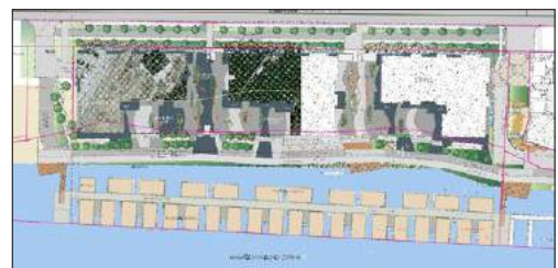
Figure 3: The water lot coverage is calculated based on the above proposed dock alignment along the Manquam Blind Channel
